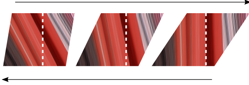
Figure 39. Calculation of Photo-Consistency. The figure shows a portion of an EPI under varying degrees of shearing. The variance along the dotted white line is minimized with the shearing slope matches the slope of the lines in the light field.
