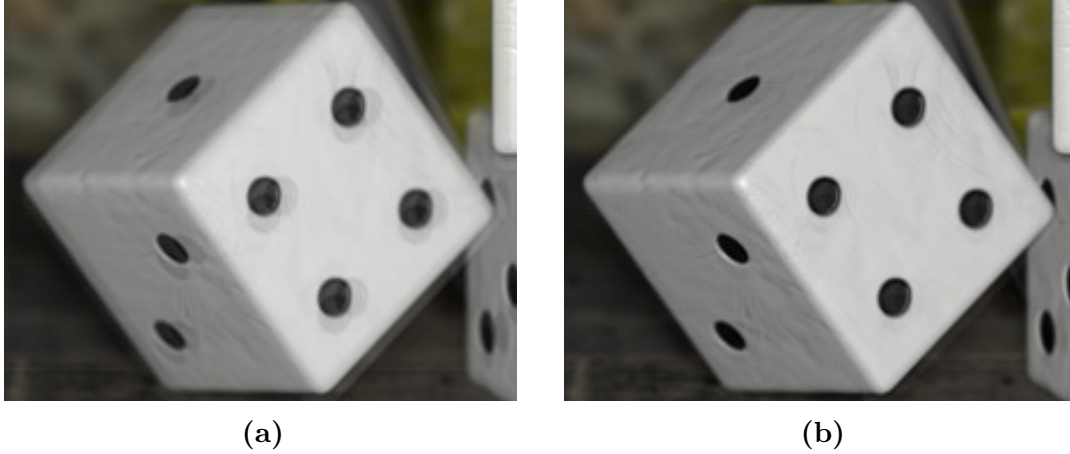
Figure 18. Refocused Image Comparison. The image formed using cubic interpolation in (a) shows noticeable aliasing near the dots and edges of the die. These artifacts are reduced considerably by using Kaiser-Bessel interpolation (b).
